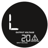
Under voltage warning
